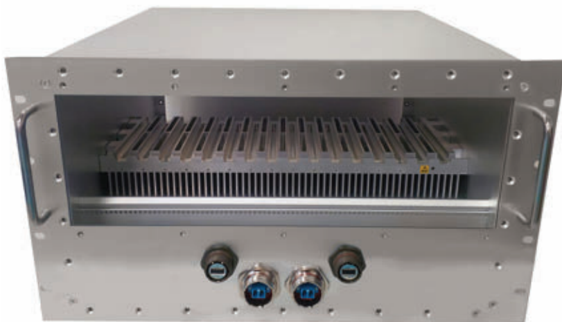
1. One way to manage faster and hotter plug-in OpenVPX boards is via a SOSA-aligned enclosure, which provides airflow over the fins of specially made conduction-cooled card mats. It can cool over 1500 W in the system. Pixus Technologies
