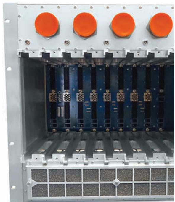
3. The VITA 48.8 specification provides for airflow to go through the modules themselves, enabling more heat to be dissipated in the system.
